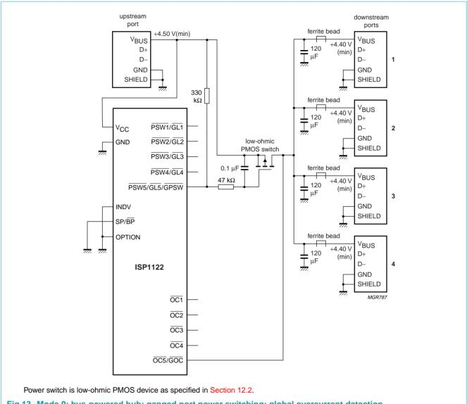
Fig 13. Mode 0: bus-powered hub; ganged port power switching; global overcurrent detection.
